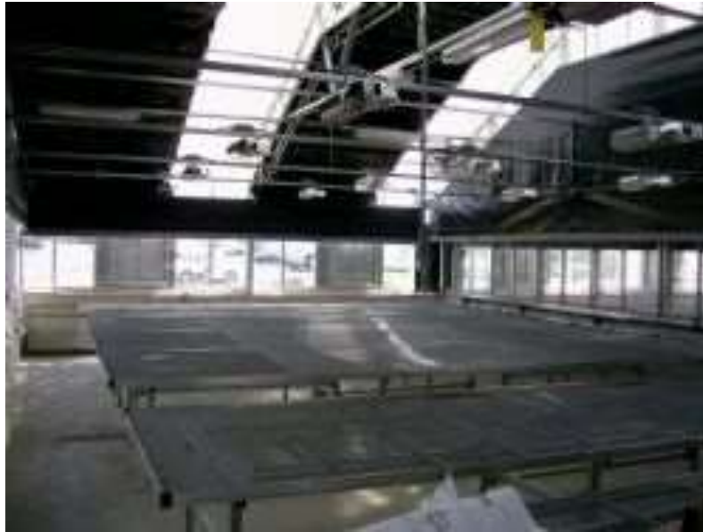
Rolling benches to reduce aisle space
